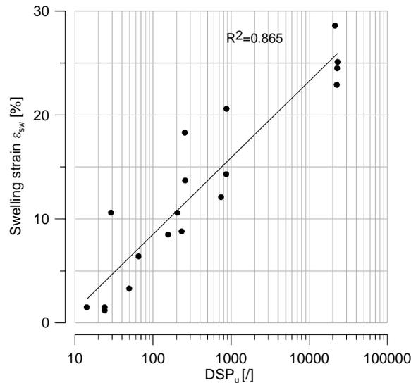
Figure 1. Evolution of swelling strain  $\varepsilon_{sw}$  vs. dimensionless parameter  $DSP_u$  for data after Villar (2000).  $DSP_u$  defined with  $a=1$ ,  $b=-2$  and  $c=1$ . 18 test results.
