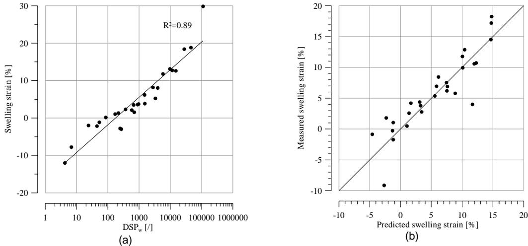
Figure 4. (a) Calibration of the dimensionless model: evolution of the swelling strain versus  $DSP_w$  for data after Yevnin & Zaslavsky (1970). Model is defined by  $\varepsilon_{sw}=3.2 \cdot \ln(DSP_w)-16.6$  with  $b=5$ .(b) Use of the model for prediction: Measured swelling strain versus predicted swelling strain.
