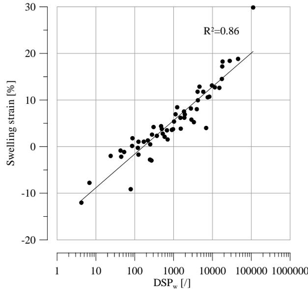
Figure 2. Evolution of swelling strain  $\varepsilon_{sw}$  vs. dimensionless parameter  $DSP_w$  for data after Yevnin & Zaslavsky (1970). 56 test results.
